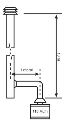
Using the information from the diagram, complete the following tables by giving the minimum size of the flue for each situation according to AS/NZS 5601 Part 1.
