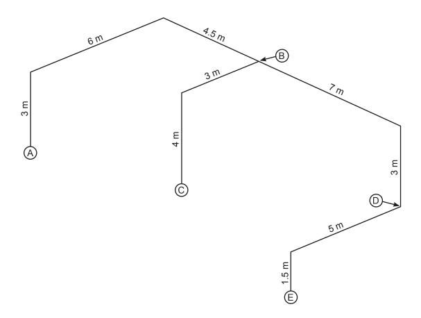
Complete the following table to show the number of clips required for the pipework. The clips are to be installed to comply with the minimum requirements of AS/NZS 5601 Part 1.
