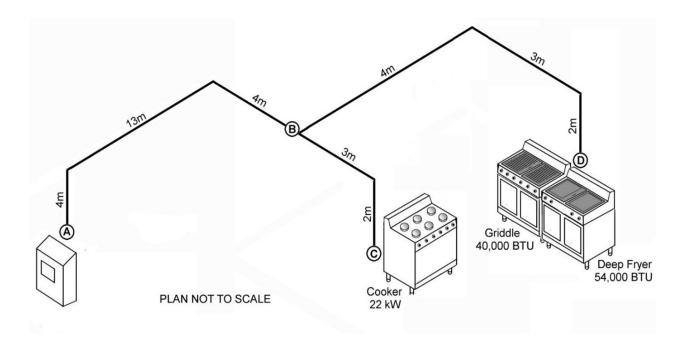
Use the Pipe Sizing Tables (not the graphs) from AS/NZS 5601 Part 1 to complete the table below.
