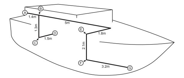
Complete the following table to give the number of supports required for the pipework. The supports are to be installed to comply with the minimum requirements of AS/NZS 5601 Part 2.
