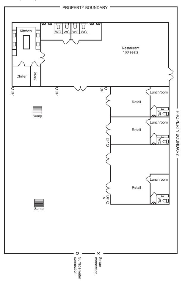
The diagram below shows the layout of a surface water drain from a sump to the Network Utility Operator's (NUO) sewer connection.
