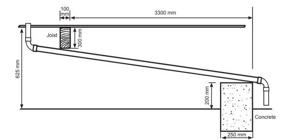
Calculate the maximum gradient achievable for the pipe without cutting the joist or the concrete.
