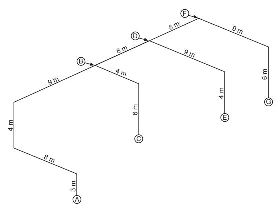
Complete the following table to give the number of clips and the rod hanger sizes required for the pipework.
