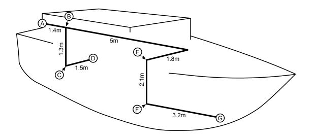
Complete the following table to show the number of supports required for the pipework. The supports are to be installed to comply with the minimum requirements of AS/NZS 5601 Part 2.
