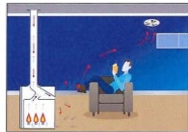
Essentially, the extraction fan can draw air from any external opening in a house like windows and doors but this can also include gas appliance flues and chimneys. This creates a problem with the operation of an open flued gas appliance, and particularly a faulty one - because dangerous gasses, such as carbon monoxide, can be drawn into living spaces from the gas appliance flue or chimney.
